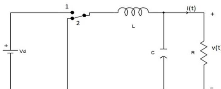
Figure.1: Basic DC-DC buck converter
