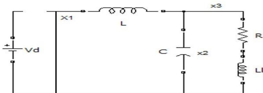
Figure 4: Buck converter equivalent circuit in OFF state
