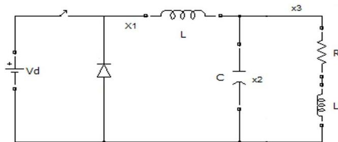
Figure 2: Buck converter with magnet load
