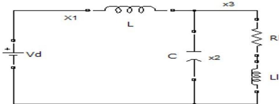
Figure 3: Buck converter equivalent circuit in ON state
