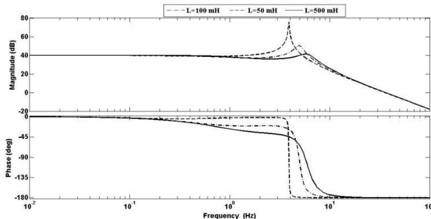
Figure 5: Frequency response of the converter transfer function for different magnet load
